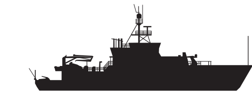
Antarctic research vessel ARANDA, ibrv, 5440 shp, d-e, built 1989
