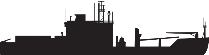
Antarctic/ Arctic research vessel AKADEMIK FEDOROV, ibrv, 16320 shp, d-e, built 1987
